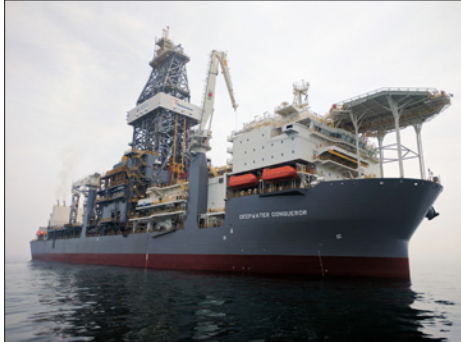
Hybrid Drillfloor installed on the Deepwater Conqueror.
